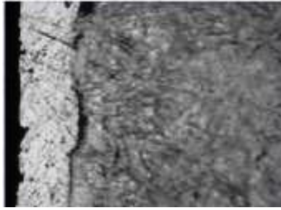
White layer developed during gas nitriding process Undesirable structure
