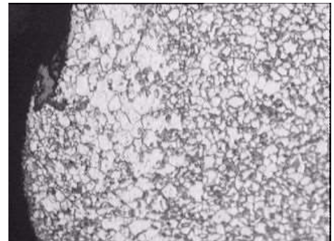
Figure 3 Shows effect of grain coarsening at OD edge on a 660MW Boiler's Water wall tube. The material of construction is SA213 Grade T22. Microstructure shows ferrite and grain boundary pearlite. (200X)
